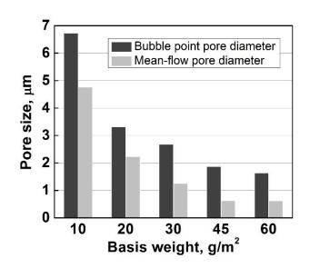
In the plot, both the bubble point and mean-flow pore diameters reduce at lower basis weights. Starting at about  $45g/m^2$ , the diameters begin to level off, in which case the minimum plateau is achieved. Hence the hypothesis is proven by the experimental results. Moreover, the mean-flow pore diameters are roughly half of the bubble point pore diameters.
