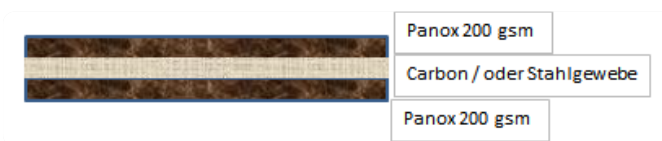
Fig. 2: exemplary, schematic representation of the structure of the oxPAN filter medium
